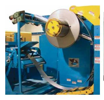
Effective coil containment is provided by a combination of hydraulic mandrel expansion, heavy-duty coil guides, and hydraulically operated hold down. The motorized endwheel is driven by an AC variable speed motor to maintain tension on the coil during payoff operations. Effective threading is provided by the hydraulic operated hold-up device designed for bottom payoff.
