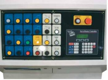
The SpaceMaster Compact Coil Line is provided with centralized controls for the entire system. The servo controls and machine controls are integrated into a sloped front control enclosure. Jog pendants are provided for functions that require the operator to access the machine. The ServoMaster Controller has a user-friendly keypad and display for job set-up and troubleshooting.
