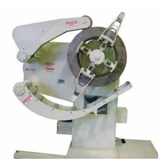
Effective coil containment is provided by a combination of hydraulic mandrel expansion, heavy-duty keepers, and air operated hold down. The motorized endwheel is driven by an AC variable speed motor to maintain tension on the coil during payoff operations. Effective threading is provided by the air operated coil hold-up device designed for bottom payoff.
