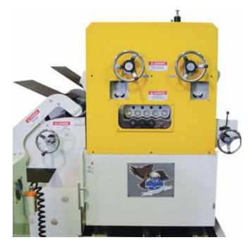
The feeder-straightener is mounted on a heavy-duty cabinet base with +/- 4" passline adjustment. The upper straightener rolls are designed with a pivoting type head for pilot release operations. The upper roll depth adjustments are made by entrance and exit side handcrank mechanisms with corresponding scales and position readouts for repeatable set-ups.
