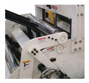
A heavy-duty funneling plate is used to catch the leading edge of the coil. The pivoting threading assist roll directs the coil into the debender roll section where coil set is removed from the strip before it is directed into the pinch rolls of the feeder. Accurate strip guiding is provided by the dual roll entrance edge guides that are mounted within the 3 roll catenary support section.
