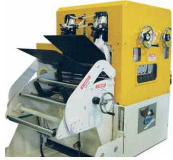
A heavy-duty funneling plate is used to catch the leading edge of the coil. The pivoting threading assist roll directs the coil into the pinch rolls. Accurate strip guiding is provided by the dual roll entrance edge guides that are mounted within the 3 roll catenary support section. The entrance pinch rolls are mounted on a true pivoting yoke mechanism and driven by a cluster gear arrangement.
