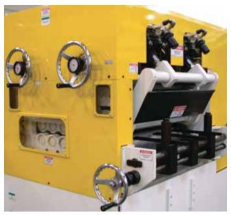
The upper straightener rolls are designed with a pivoting type head for pilot release operations. Accurate strip alignment to the press and tooling is assured by single roll exit edge guides. The feed rolls are mounted on a true pivoting yoke mechanism and driven by a cluster gear arrangement. This design assures full engagement of the drive gearing regardless of material thickness.
