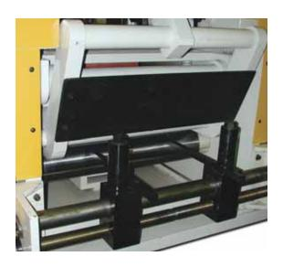
Accurate strip alignment to the press and tooling is assured by single roll exit edge guides. An offset feature of +/-1" is provided to allow adjustment of the strip position. The feed rolls are mounted on a true pivoting yoke mechanism and driven by a cluster gear arrangement. This design assures full engagement of the drive gearing regardless of material thickness.
